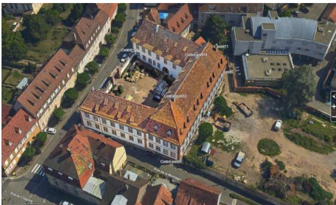
Figure 6: Selecting control points in the aerial 3D model for fine adjustment of the UAV data
