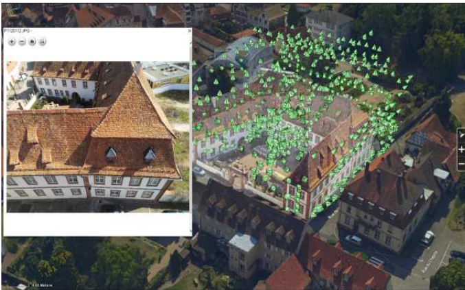
Figure 5: Results of the image orientation process on the UAV data, performed on the Palais Stanislas in Wissembourg. The camera positions are displayed.
