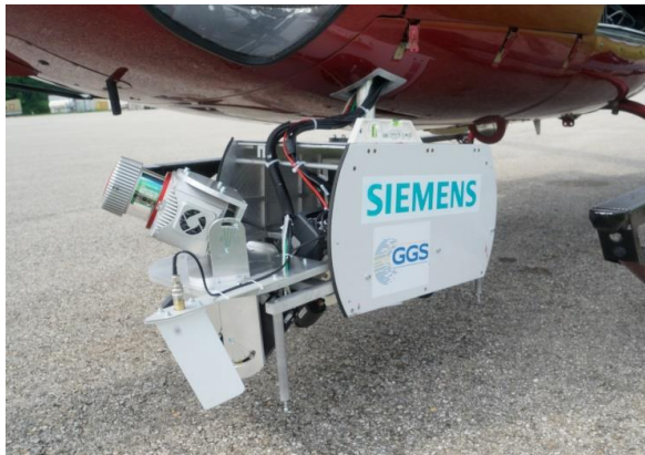
Figure 2. Sensor-head mounted on a helicopter.
